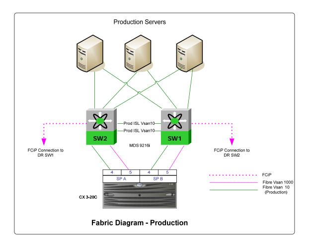
Note that CX3-20C comes with 8 iSCSI and two fibre channel front end ports. 0, 1, 2, and 3 ports are iSCSI on both SPs. Ports 4 and 5 were fibre front end. SPA5 and SPB5 were connected to a different VSAN to segregate MirrorView ports from production traffic. Production HBAs and FA ports were connected to VSAN10, and VSAN1000 was used for remote replication.
