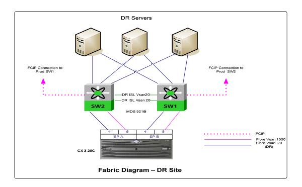
The VSAN 20 at DR site segregated Production and DR fabrics. Only VSAN1000 was allowed over FCIP to extend and merge with production. Other configurations remain the same as in the primary site.
